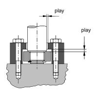
If the Safety Catcher is firmly bolted to the machine frame, the retaining rod must have sufficient play at its attachment, so that the lateral or tilting movements of the slide will not create lateral forces to the rod.
