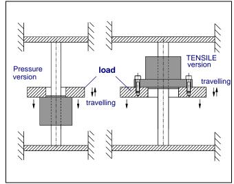
Fig. 4: Attachment options for mobile Safety Catcher
