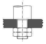
The mounting flange as shown above is one of the common solutions for a mounting with radial play. Alternatively a spring base is recommended, which on top provides additional advantages as descibed in "Technical Data Sheet TI-A20".
