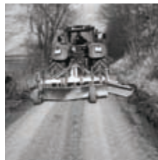
Gravel road finisher with HKS XtraTilt
